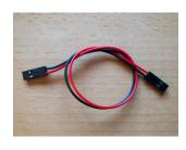
A DuPont header connection cable is included. This plugs into the motor connector. Remove the header from the other end if necessary and solder the cable to your motor lugs. If the loco goes the "wrong" way in forwards/reverse you can swap the polarity of the cable.
