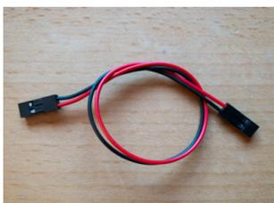
A DuPont header connection cable is included. This plugs into the motor connector. Remove the header from the other end if necessary and solder the cable to your motor lugs. If the loco goes the “wrong” way in forwards/reverse you can swap the polarity of the cable.
