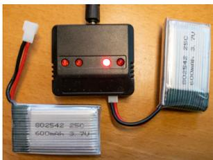
The standard way to charge the Lipo battery is to remove it from the loco and use the mini charger supplied with the batteries. The LED is on while the battery is charging and goes off when completed. Having a spare charged battery also means the loco can quickly be up and running again after the initial battery runs down.
